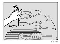
**2** While pushing the release button, lift the ADF unit.
