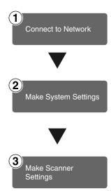
Connect the machine to the network with an Ethernet cable or IEEE 1394 (optional) cable, or use Wireless LAN (optional). See *Network Guide*.
