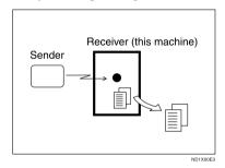
Normally this machine receives messages by Immediate Reception, but Memory Reception is used with the following function:
