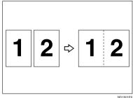
Two A5 ☐ messages are printed side by side on a sheet of  $A4\square$ .
