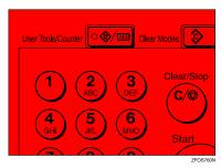
Press the ③ or ⑤ key to display "3. Copier Features", and then press the [OK] key.
