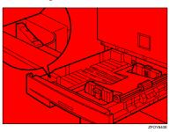
While pressing the release lever, adjust the side fences.
