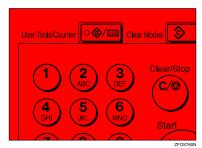
Press the ③ or ⑤ key to display "2.System Settings", and then press the [OK] key.
