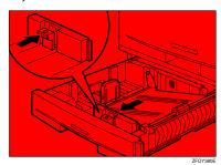
Push the metal plate down, and then square the paper and load it in the tray.
