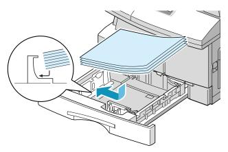
You can load letterhead paper with the design side facing up. The top edge of the sheet with the logo should be placed at the right side.
