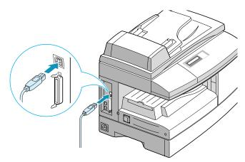
If you want to use a parallel printer cable, only use a IEEE 1284 compliant cable and connect it to the parallel connector on your machine.
