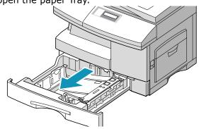
**2** Push down on the pressure plate until it locks in position.
