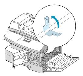
**6** Turn the Jam Remove Lever back to the original position.
