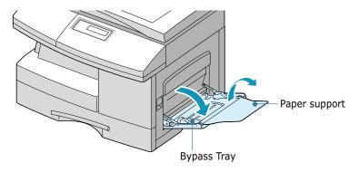
**2** Prepare a stack of paper or envelopes for loading by flexing or fanning them back and forth. Straighten the edges on a level surface.
