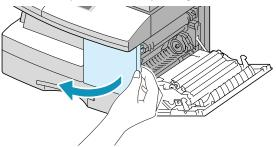
**2** Turn the cartridge locking lever upwards to unlock the toner cartridge, then pull the toner cartridge out.
