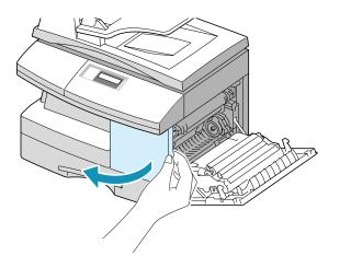
**3** Pull down on the fuser lever. This will release pressure on the paper.
