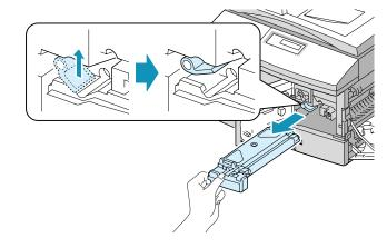
**NOTE:** The toner cartridge must be removed to replace the drum cartridge.
