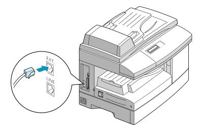
**NOTE:** You should use the telephone line cord which is supplied with your machine. If you are replacing it with another vendor's, it should be AWG #26 or lower gage.
