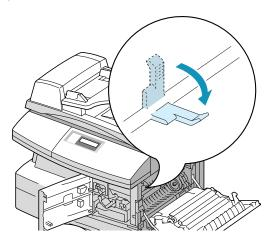
4 Turn the Jam Remove Lever in the direction of the arrow to move the paper to the exit area, then gently pull the paper out through the exit area.
