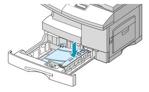
**3** Adjust the rear paper guide to the desired paper length. It is preset to Letter or A4 size depending on the country. To load another size, lift and insert the rear guide into the corresponding position.
