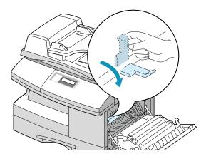
**WARNING:** The fusing area at the rear part of the inside of your machine is hot when powered.Be careful not to be burned when you access this area.
