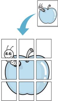
This special copy mode can be applied when you load document only using the document glass. If a document is detected in the ADF, the Poster copying feature does not work.
