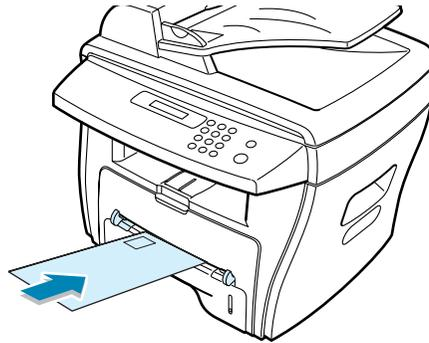
2 Adjust the paper guide to the width of the print material.
