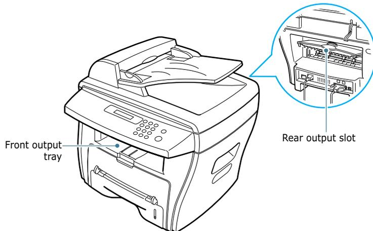
To use the front output tray, make sure that the rear cover is closed. To use the rear output slot, open the cover.
