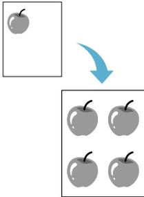
This special copy mode can be applied when you load document only using the document glass. If a document is detected on the ADF, the Clone copying feature does not work.
