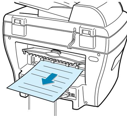
Printing from the Bypass tray to the rear output slot provides the **straight paper path**. Using the rear output slot might improve the output quality with the following:
