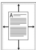
This special copy mode can be applied when you load document only using the document glass. If a document is detected in the ADF, the Auto Fit does not work.
